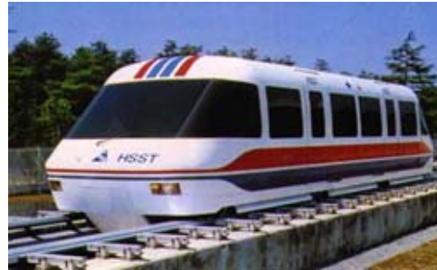
Figure 10-38: Maglev vehicle with linear induction motor propulsion. (HSST Corporation)
