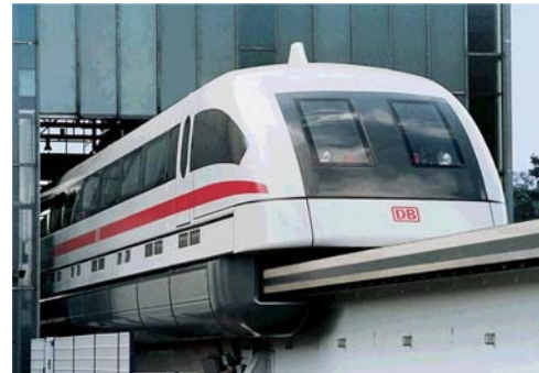
Figure 2-7: Advanced transport system with magnetic suspension. (Transrapid International)
