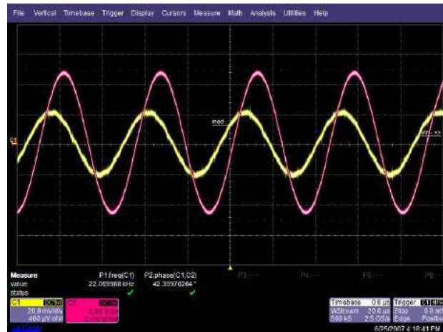
Figure 8.4: OPA227 A_v=50\text{dB} @ 22 kHz
