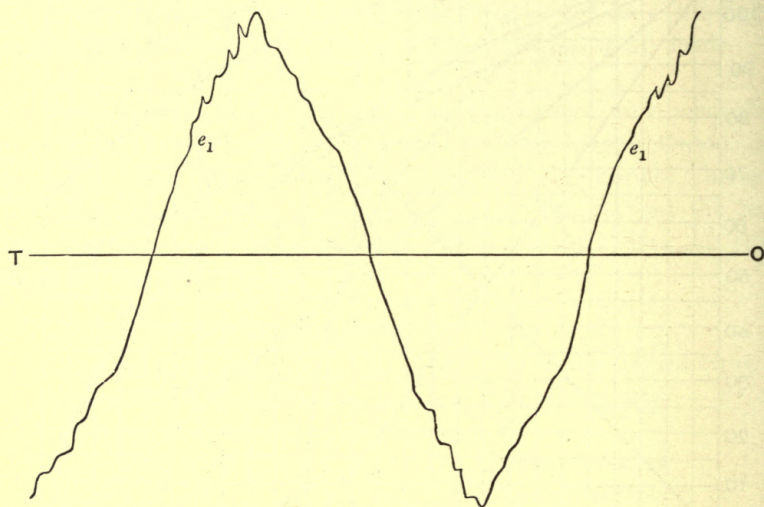
Fig. 60. Shape of the electromotive force wave of a two phase machine on open circuit.
