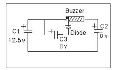
If you want to check it out, here is the circuit. C1 and C2 are electrolytic capacitors with 4700 uf each. C3 is an electrolytic capacitor with 470 uf. For the diode any universal diode with appropriate working voltage will do it. I used (DRR 104). The buzzer is self-made from an old telephone-ringing coil and the contacts are from an old relay.
