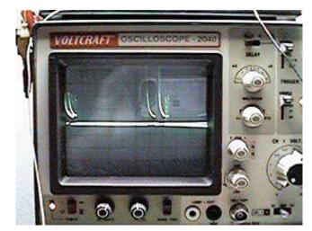
This is the typical image of back-EMF. The voltage spikes are more than 4 squares up, each square means  $5 \times 10$  volts (due to  $10 \times 10$  probe). Certain tingling in fingers is felt when touching the blank wire. If it were not for the low amperage in this circuit the 200 volts spikes would have been dangerous indeed. All this from a buzzer at  $10 \times 10$  volts and  $3-4 \times 10$  mA(DC).
