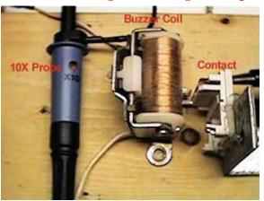
The picture shows: A 10 x probe which is reducing incoming measuring voltage for an oscilloscope. An electric coil (~1 k ohm resistance) from an old phone bell with buzzing mechanics operating a contact which is made from an old relay (coil removed). Back EMF is what you get when an electric current stops
