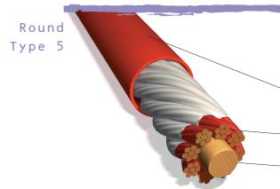
Type 5 Litz construction features insulated bundles of Type 2 Litz wire twisted around a fiber core.
