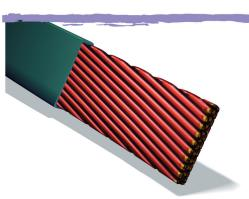
Many Litz wire constructions are available with multiple layers of insulation to meet the voltage-withstand requirements of UL and IEC. Multiple extruded layers of fluoropolymers, such as FEP, PFA, and ETFE are most common. These extrusions are offered in different colors so that the different layers are easily distinguishable.
