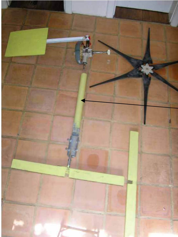
3 inch galvanised steel pipe pole
